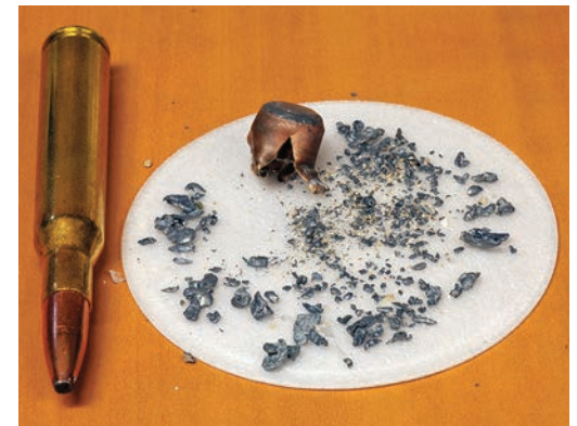
Lead particles show up as white flecks (top) in this X-ray of viscera taken from a euthanized sheep that was shot as part of a DNR study of lead bullet fragmentation. When fired into a series of water jugs, the lead in a standard copper-jacketed bullet (above) splinters into shards and fine particles.
