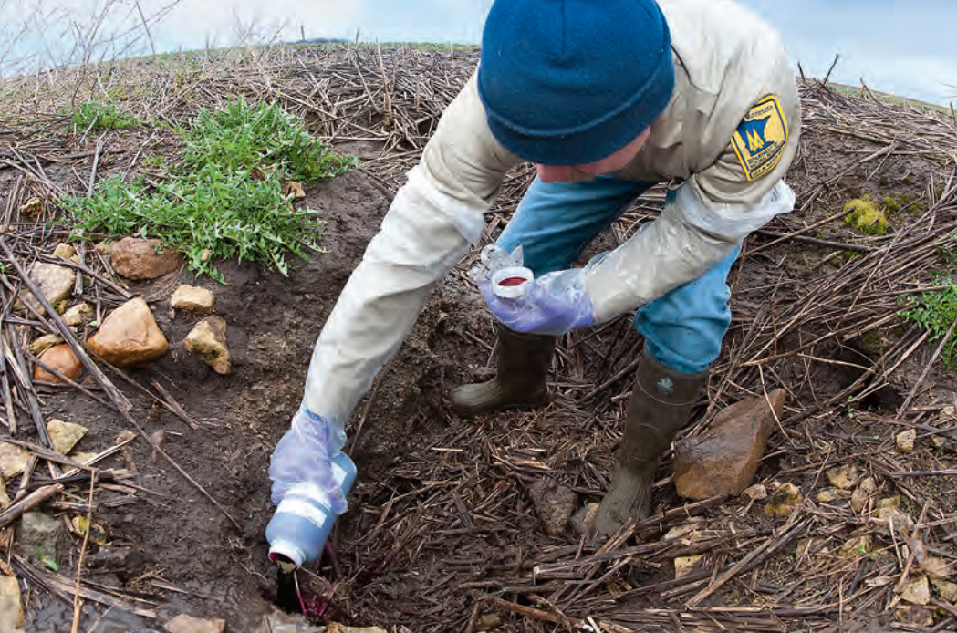
A dye trace begins when a nontoxic organic dye (above) is poured into a sinkhole or other karst feature. Water is then used to flush the dye into the sinkhole. Springs in the area of the sinkhole are monitored for traces of the dye.
